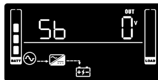
Figure 17: Display in standby mode
